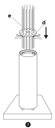
The speaker cable are fastened to spring so the cable always straight. The 12 speaker cable need to be connected to the Trunk electronics
